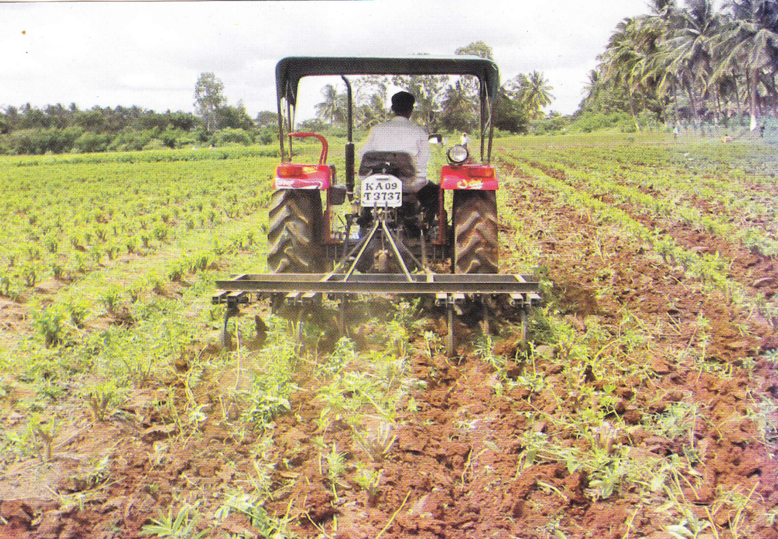
Figure 3.30 : Intercultural operations in a mulberry garden by a tractor operated cultivator (a) 7 days after pruning (b) 25 days after pruning
