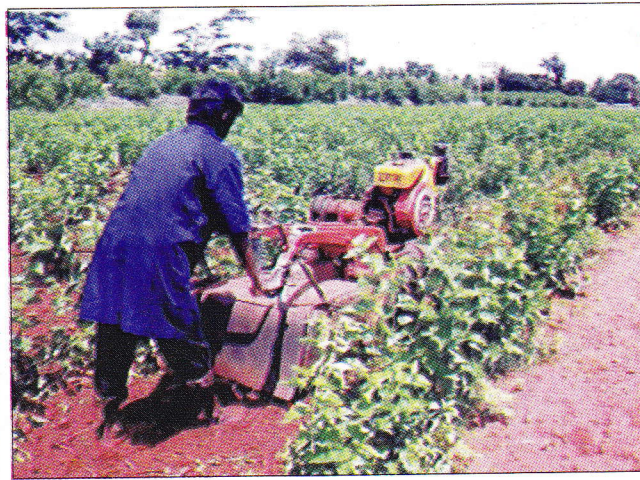
Figure 3.28 : A power tiller operated rotavator in a mulberry garden
