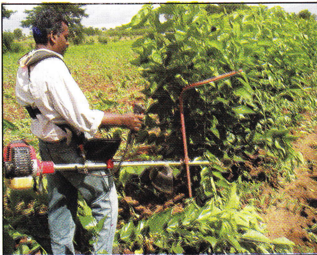
Figure 4.3 : Knapsack type bush cutter/ pruner and mulberry shoot harvesting with it.
