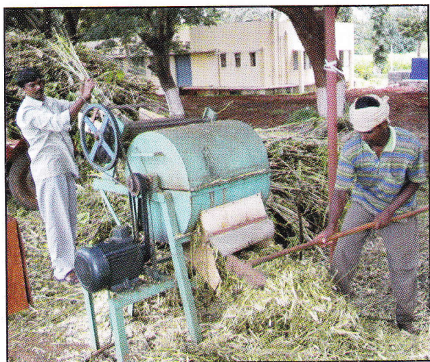
Figure 4.4 : Shoot Crushing machine in operation and heaps of crushed mulberry shoots for composting
