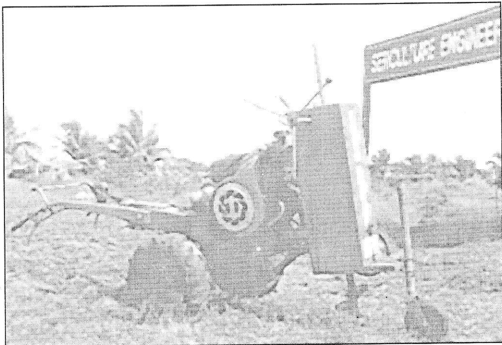
Figure 3.9: A power tiller operated auger digger
