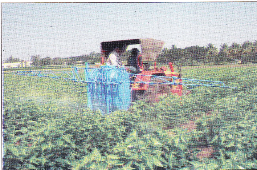
Figure 3.42 : (a) Self Propelled sprayer (b) Power tiller mounted sprayer (c) Tractor mounted sprayer
