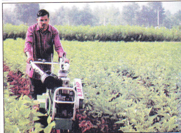
Figure 3.29 : Different types of self-propelled weeders
