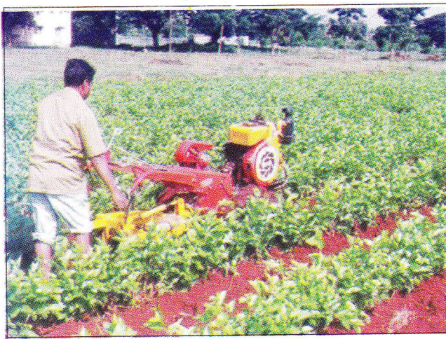
Figure 3.27 : A power tiller operated cultivator in a mulberry garden
