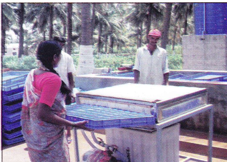
Figure 4.13 : Plastic tray washing machine
