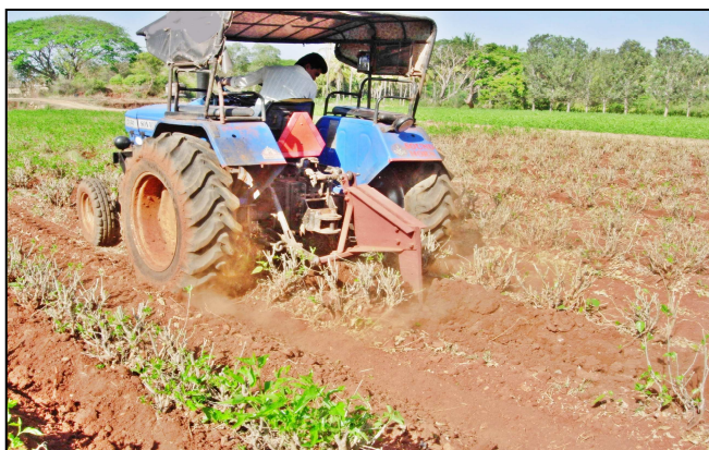
Figure 3.18: A subsoiler operating in a mulberry garden for loosening the subsurface soil to increase water infiltration and water holding capacity of
