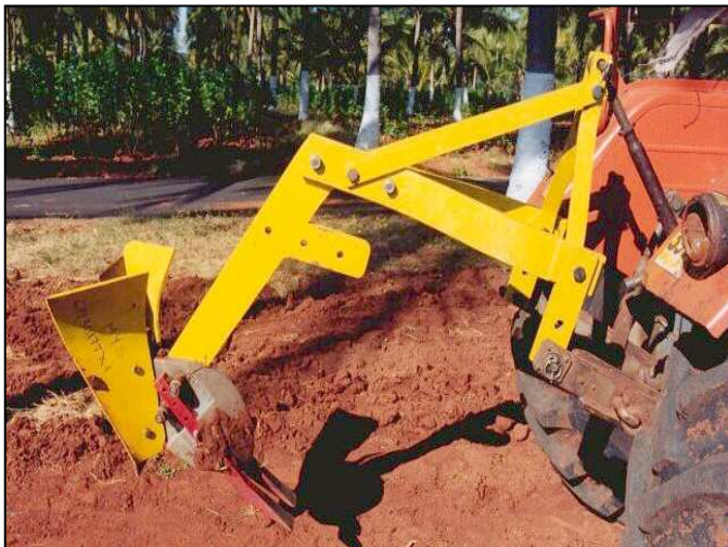
Figure 3.8: A tractor operated trencher
